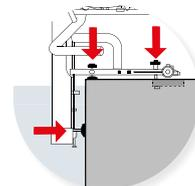
Screw in the fixing shaft and adjust the height of the adjustment feet.
